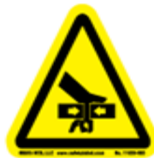
Hand Crush/Force from two sides
